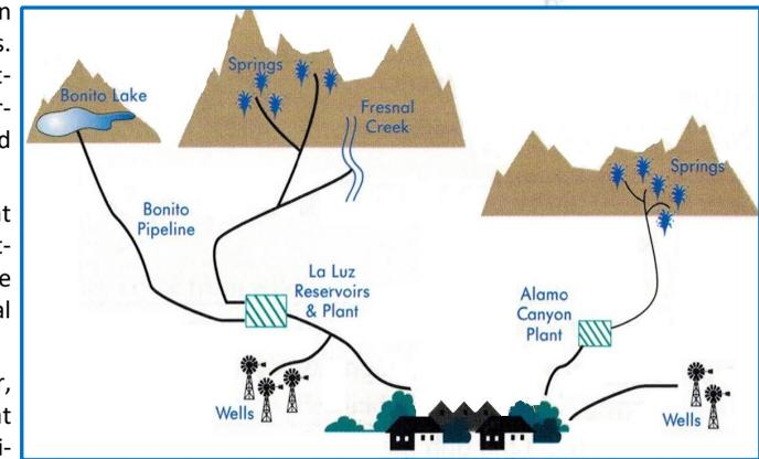
collected from these areas is piped to the City's 188 million gallon raw storage and treatment facility in La Luz. The water is then filtered and disinfected then gravity flows to our customers. On the southern
